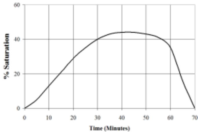
Using more salt than necessary. Reduce brine draw to save salt
