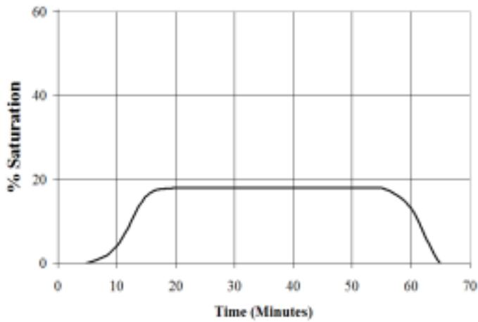
Brine eductor, a device that uses flowing water to draw brine out of the brine tank, draws too slowly. It should be adjusted to draw brine faster
