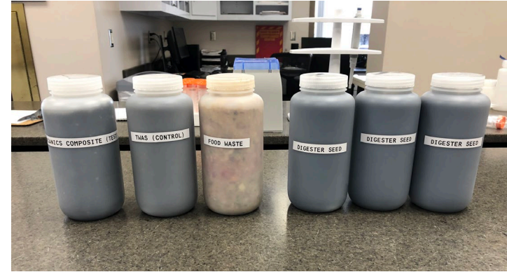
Figure 8: Biomethane Potential (BMP) samples from the food pilot.
