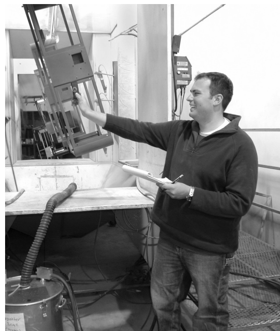
The MnTAP intern at Ultra Image tested the air flow in the powder coating booth to determine transfer efficiency.
