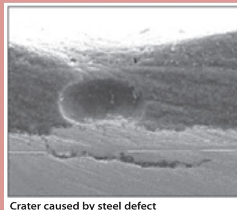
Crater caused by steel defect
