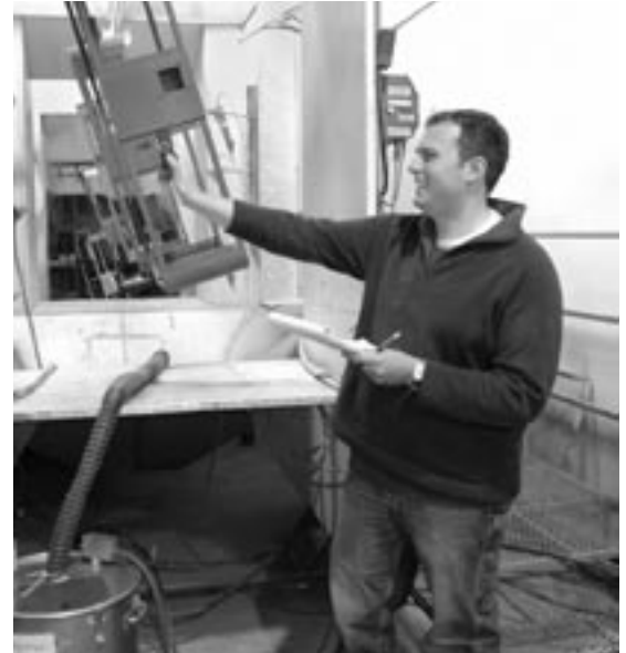
The MnTAP intern at Ultra Image tested the airflow in the powder coating booth to determine transfer efficiency.
