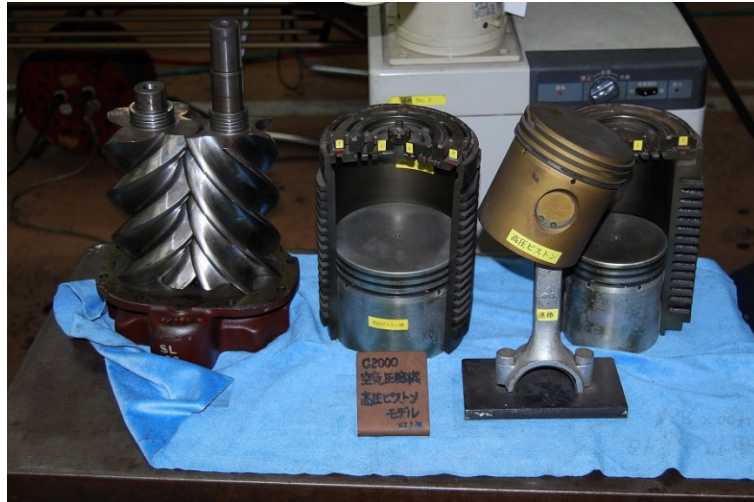
Figure 1 Piston type compressor on the middle and rotary screw compressor on the left.
